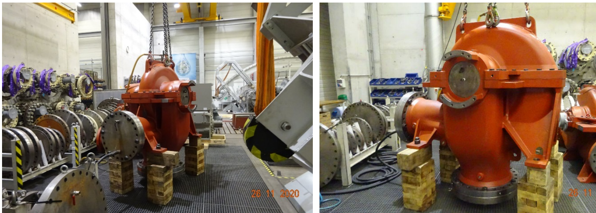
Figures 6a and 6b: Factory Acceptance Testing of the new high lift pumps was completed at the KSB factory in Halle, Germany. This testing confirms the pumps will perform as specified prior to being shipped to site.
